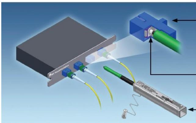
Illustration of cleaning procedure for SC connectors
